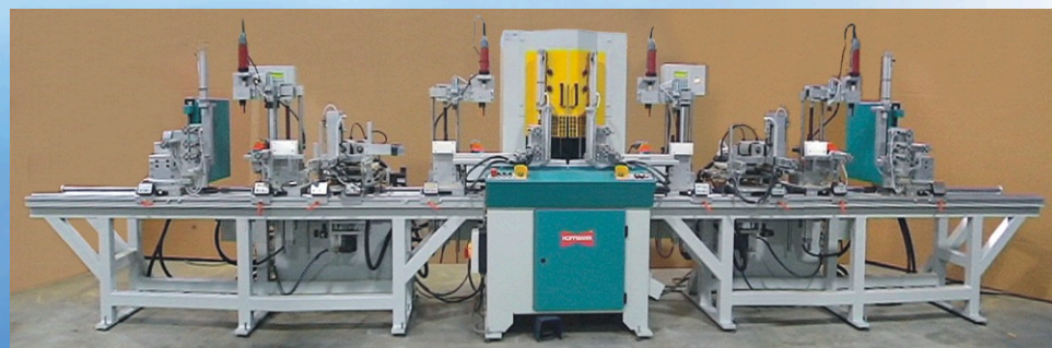
The Door-set machining centre "ZBZ 5" processes, in five machining sequences, everything necessary for each door-set. The parts are simultaneously machined in pairs.
