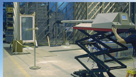
The fixed glazed "Hoffmann Window" was hit with a 2.5m long roofing lath, which was fired from a high pressure air cannon.
